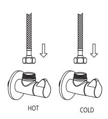
4. Finally, connect the cold and hot water inlet hose to the valve of supply water and finish installation. Please must pay attention to open the valve to clear the sundries in the pipe before connectting the valve from being blocked.
