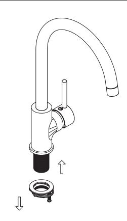
1. Rotate the screw tube and install into the faucet ,then remove the nut and gasket.
