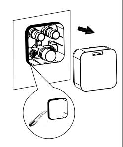
$3. \\ After decorating the wall, remove the protective cover and divide the part of the concealed box above the wall.$
