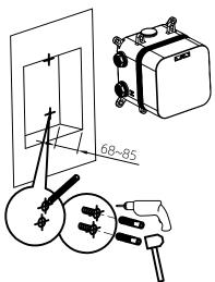
1. According to the picture of mixer instrallation size,dig a suitable hole in the wall (the depth of the wall is 73-86 after decoration). Put the mixer in the
