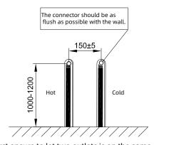
First ensure to let two outlets is on the same level before instrallation and the distance between two water outlets is within the allowable range. Please use the left-hot right-cold connection for the cold and hot water.
