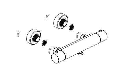
Screw into decorative cup and then the hex nut on the mixer. Fix the main body to the water inlet connector.
