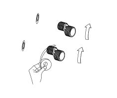
After wrapping the eccentric with PTFE tape,please connect with the pre-embedded water oulet pipe connector.
