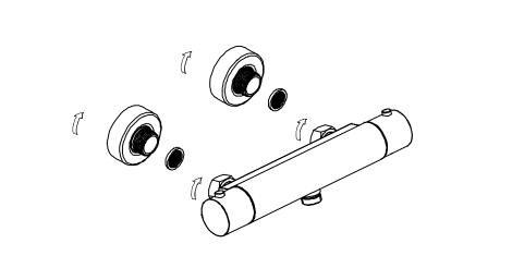
Screw into decorative cup and then the hex nut on the mixer. Fix the main body to the water inlet connector.
