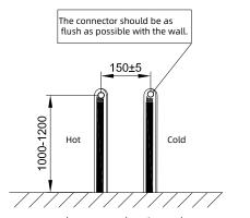
1. First ensure to let two outlets is on the same level before instrallation and the distance between two water outlets is within the allowable range. Please use the left-hot right-cold connection for the cold and hot water.
