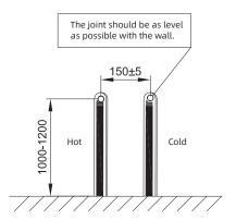
1. First ensure to let two outlets is on the same level before instrallation and the distance between two water outlets is within the allowable range.Please use the left-hot right-cold connection for the cold and hot water.
