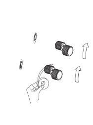
After wrapping the eccentric with PTFE tape, please connect with the pre-embedded water oulet pipe connector.
