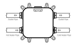
2.Use your own water pipes connections, connect the mixer to the hot and cold water sources by the left hot (red) right cold (blue)(not and cold water must be connect correctly, otherwise the temperature cannot be adjusted). The water outlet is connected to the required water outlet port respectively(shower head, hand shower, etc) and check any leaks at each connection.
